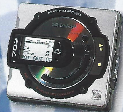
➤ Sharp and Sony introduce portable MiniDisc recorders. This digital alternative to audiocassettes records customized music compilations and doesn't skip when bumped.
